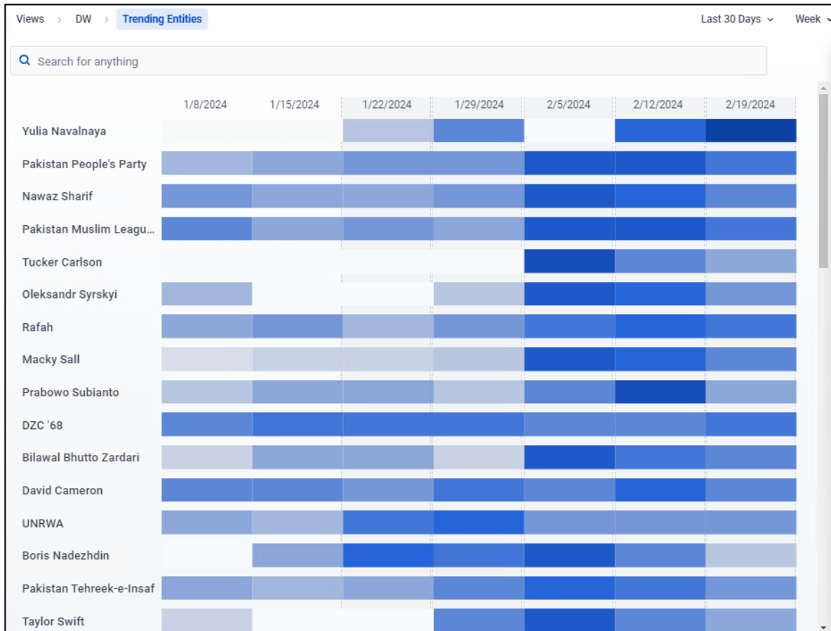
Figure 2 Named Entities (linked to Wikipedia), as detected by the Named Entity Recognition and Linking model developed within SELMA, trending in a date range of 30 days. Entities are considered to be “trending” according to a “pointwise mutual information” criterion ( https://en.wikipedia.org/wiki/Pointwise_mutual_information ).
